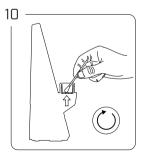
Use a cotton swab or Dual Tool to clean the chamber after each use. Wipe gently in a circular motion.
