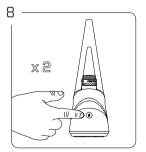
Double click to initiate heat-up. Press and hold button anytime to exit. Pulsing light indicates heat-up mode is active.
