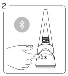
Hold the button for 6 seconds to sync your Peak Pro with your app. The device will turn on/off, keep holding until glows blue.
