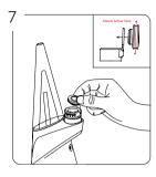
Place carb cap on top of chamber. Press down until snug. Use the included chamber jacket  $\theta$  tether to keep it safe during use.
