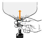
Detach Valve Balloon from Filling Chamber
