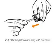
Disassembling the Filling Chamber
