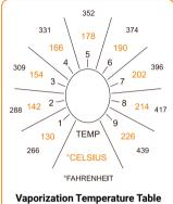
The vaporization temperature may fluctuate about ± 5°C (± 9°F) related to the indicated values because of the heating and cool off process of the heat exchanger. For example at level 6 from 185°C up to 195°C (365°F up to 383°F).
