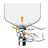
Detach Valve Balloon from Filling Chamber
